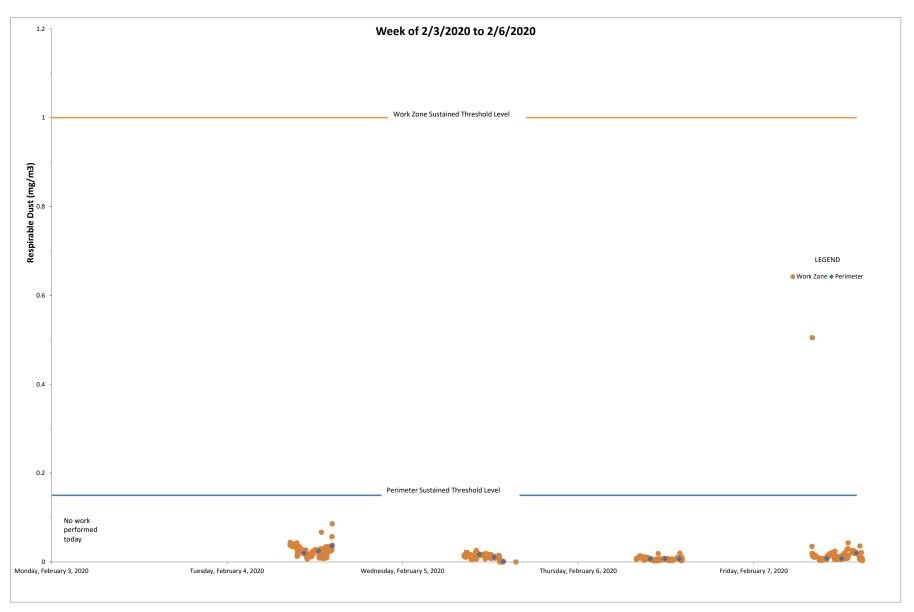
Transient readings were conducted over a three minute time period. A reading is sustained if it is held for over a five minute time period.
